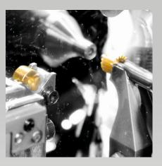
All our machines are equipped with Affolter Leste CNC-Controls. which can control up to 12 axes. The interpolation speed is 90 ns! This proprietary control design affords unique speed and machine dynamics.
