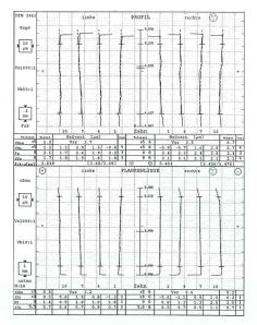
3 Measuring log of a gearwheel with a module of 0.35, helical–toothed with  $\beta$  11.5°, hardness 61 to 63 HRC finishmachined with skiving on a Gear AF100
