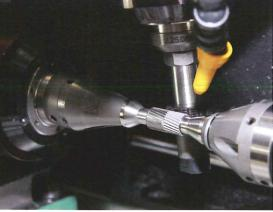
2 The  $\mu$ -skiving technology enables high-precision manufacturing of gearwheels in the module range from 0.1 to 1.0 with the skiving method
