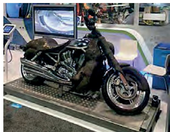
Dry-ice cleaning allows items to be cleaned in place without disassembly. (Courtesy: Cold Jet®)
